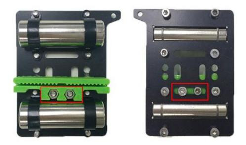
Step3. Fix the extruder holder on the front side of the X carriage using M4x6mm screws.
