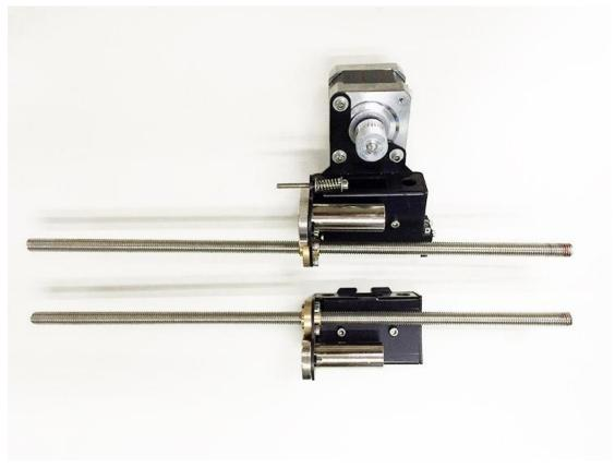
Step2. Plug the threaded rod on the X motor end to the left coupling on the left bottom of the Z axis. Then thread the 320mm smooth rod into the linear bearing.
